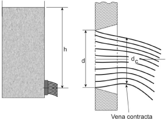
At the vena contracta, the volumetric flow rate Q of the fluid is given by
